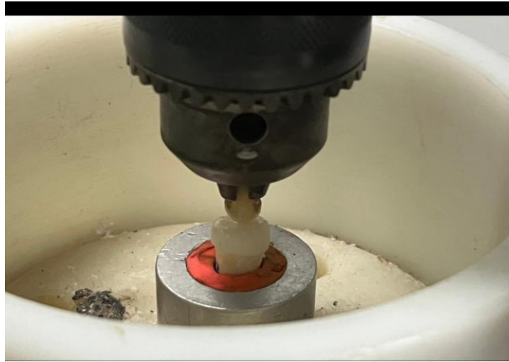
Figure(1) Chewing simulator utilized for wear test
