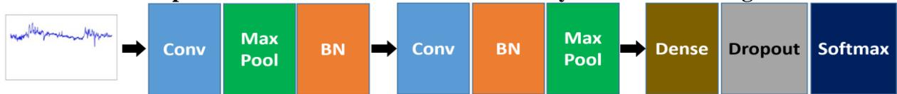
Figure 4: The 2-layer Convolutional Neural Network.
