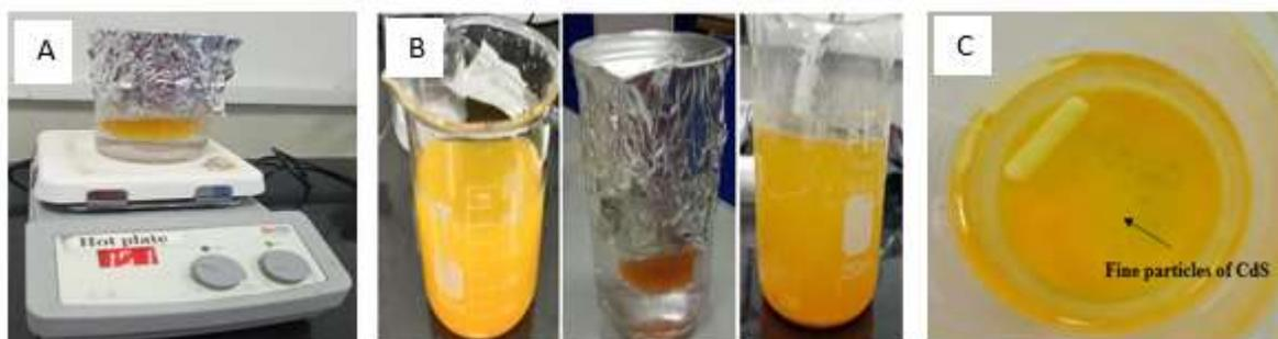
**Fig.1** Synthesis of Cysteine Capped Cadmium Sulfide Quantum Dots (A) and (B) CdS QDs synthesis by using chemical method in beaker by using hot plate (C) Cadmium sulfide quantum dots at the bottom of beaker
