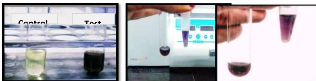
**Fig.2** Ninhydrin test to check the binding of cysteine with CdS QD
