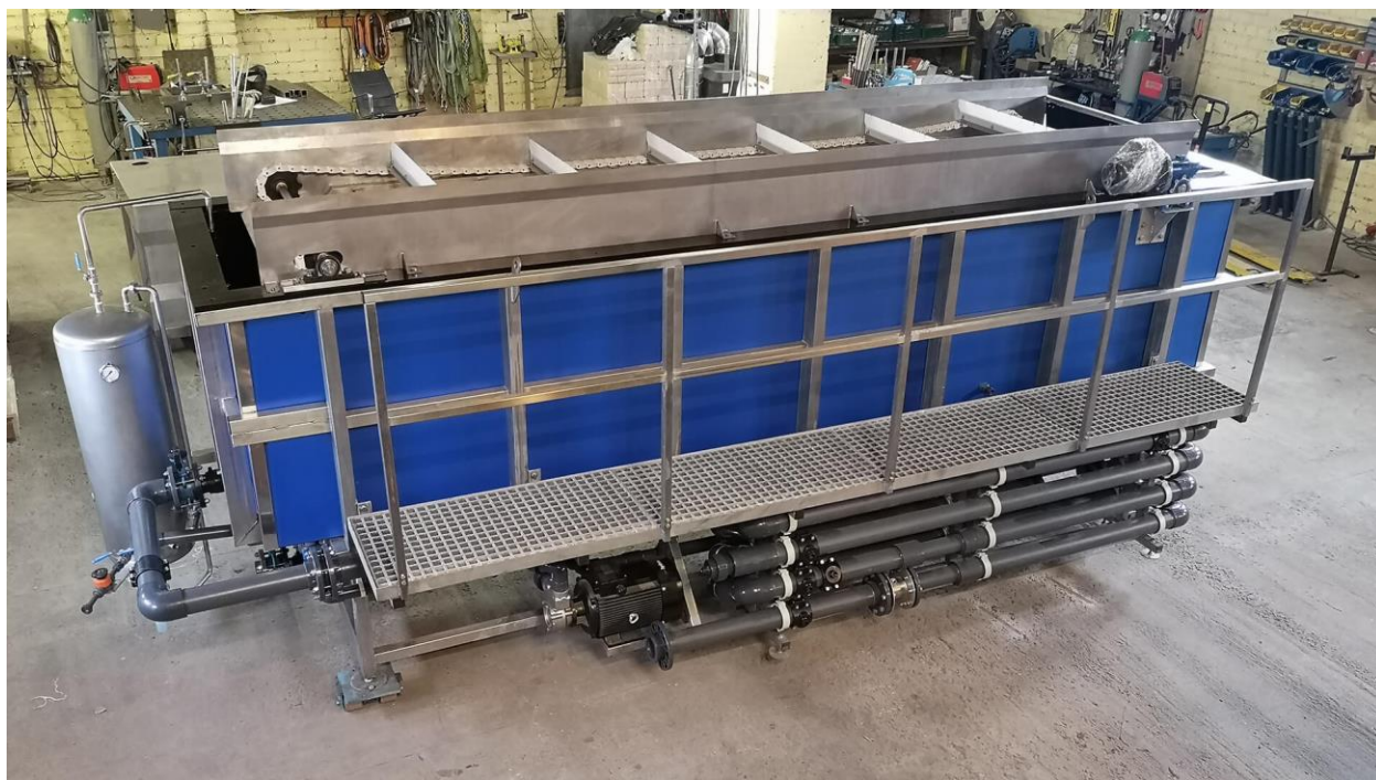
Figure 1 – Dissolved air float at the Riograndense oil refinery.
