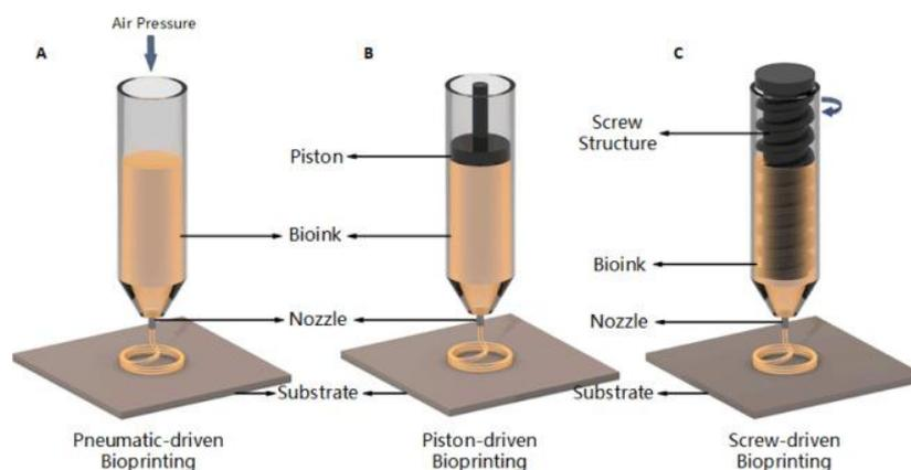
**Figure 5:** shows a schematic illustration of the three common extrusion-based bioprinting techniques (a pneumatic, b piston, and c screw).
