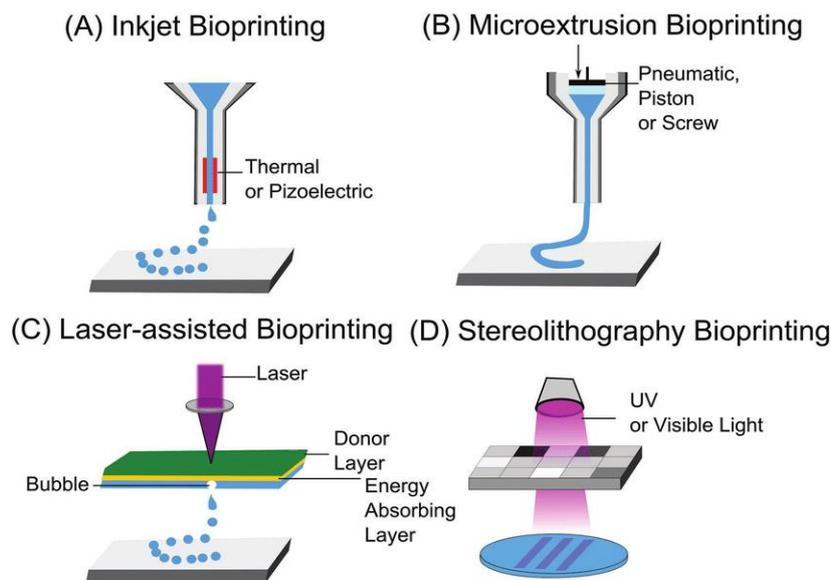
**Figure 3.** Methods for bioprinting. To create tissues, the inkjet bioprinter progressively ejects tiny droplets of hydrogel and cells. The extrusion bioprinter continuously extrudes a liquid cell hydrogel solution using pneumatic or manual force. c A laser printer's positioning diagram. D Diagram of the dynamic optical projection stereolithography (DOPsL)-based bioprinter.
