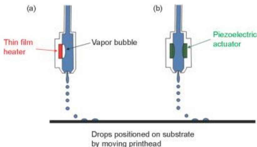
**Figure 4:** Schematic diagram of the inkjet printing technique that uses piezoelectric and thermal actuators for on-demand printing. Using a heating component to increase the temperature locally and produce a bubble that forces droplets through the nozzle, a thermal print head works. When voltage is applied, a material that changes shape and expels droplets is used with a piezoelectric head.
