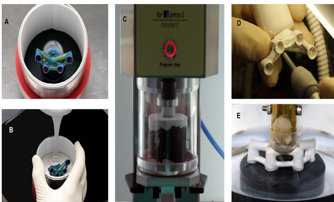
Fig. 2. Steps of construction and testing of the PEEK frameworks; A: The wax pattern fixed in the investment mold; B: Pouring of the investment material before placement into the furnace; C: The mold containing the melted BioHPP in the pressing unit; D: The remaining investment material removed by air-abrasion; E: The specimen fixed and tested for retention in the chewing simulator.
