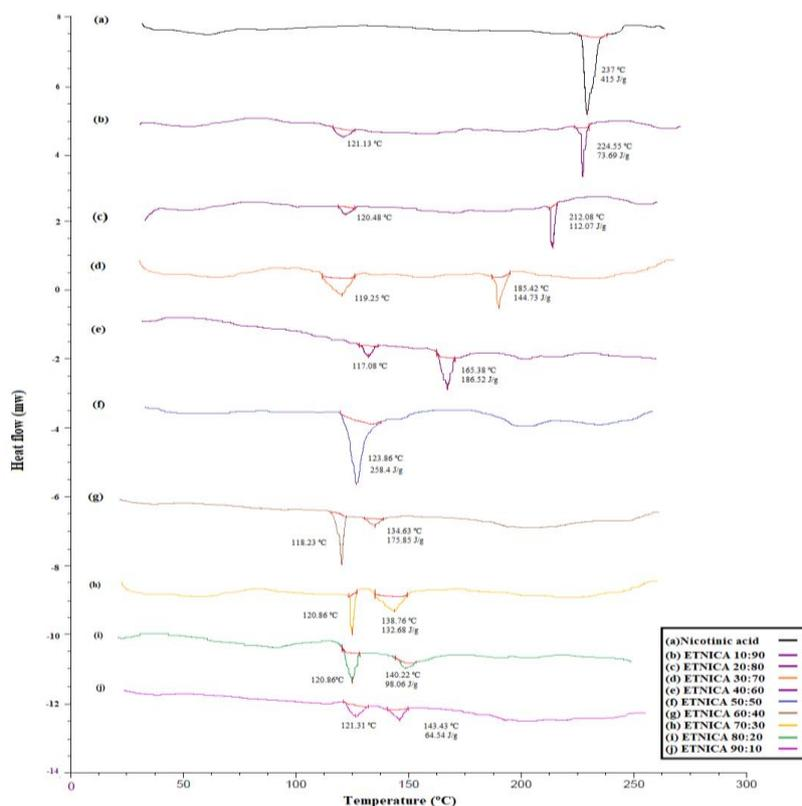
**Figure 6: DSC thermograms of nicotinic acid and all compositions of ETNICA Binary phase diagrams.**
