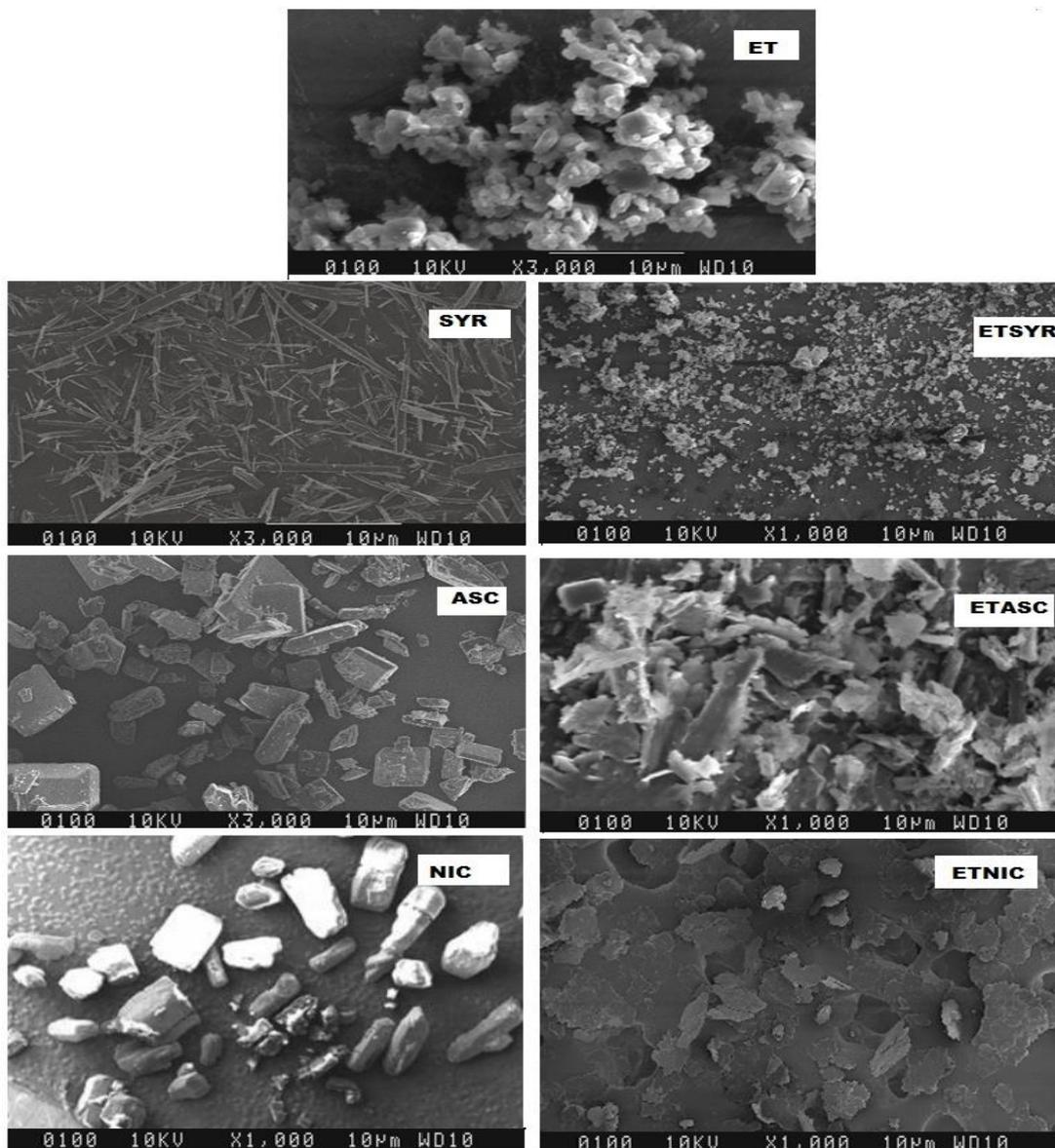
**Figure 18: Scanning electron microscopy images of Etodolac (ET), Coformers (SYR, ASC, and NIC), and corresponding eutectics (ETSYR, ETASC, and ETNICA)**
