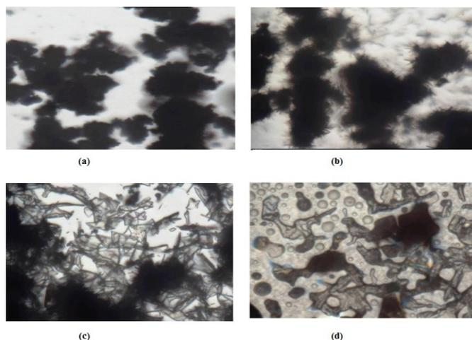
**Figure 14: ETASC before melting, (b) ETASC starting to melt, (c) ETASC melting at 123.86°C and (d) ETASC fully melted**
