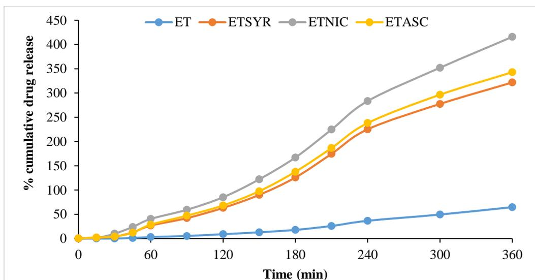
Figure 20: Dissolution profile of etodolac and its respective eutectics
