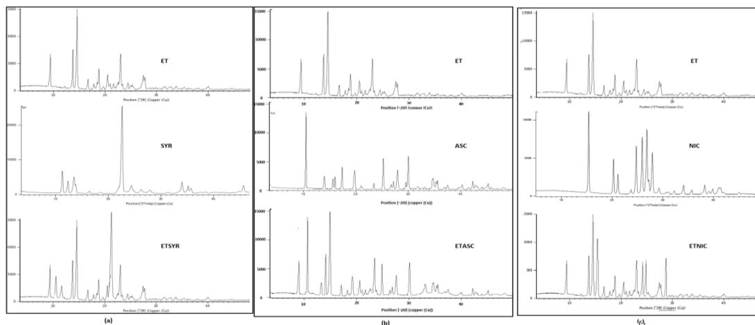
**Figure 17: PXRD pattern of Etodolac (ET), Coformers (SYR, ASC, and NIC), and corresponding eutectics (ETSYR, ETASC, and ETNICA)**
