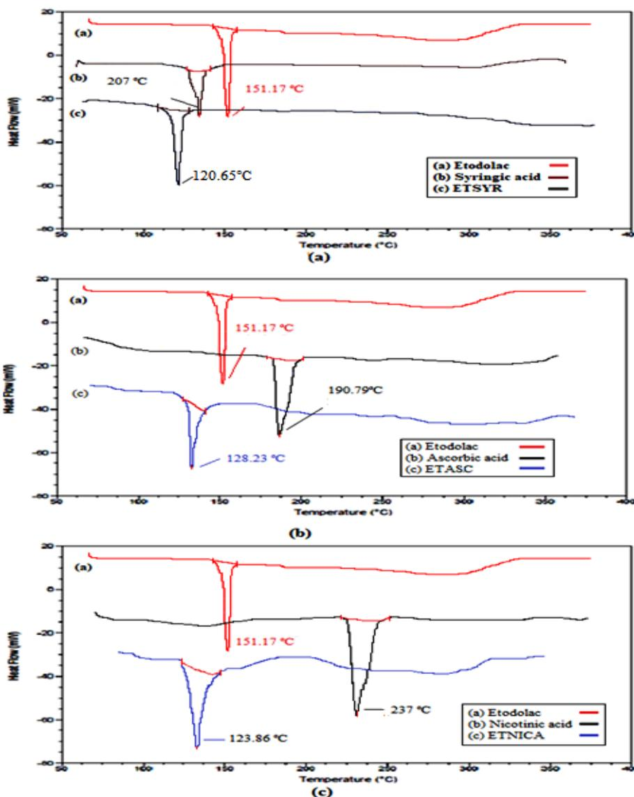
**Figure 3: DSC thermograms of (a) ETSYR (b) ETASC (c) ETNICA**
