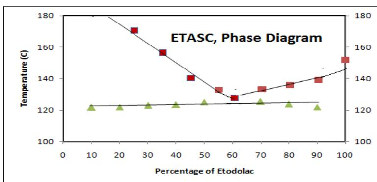
Figure 8: Binary phase diagram of ETASC
