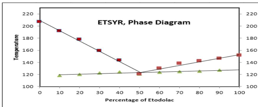
Figure 7: Binary phase diagram of EYSYR
