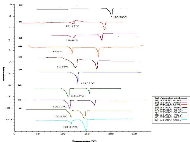
**Figure 5: DSC thermograms of ascorbic acid and all compositions of ETASC**
