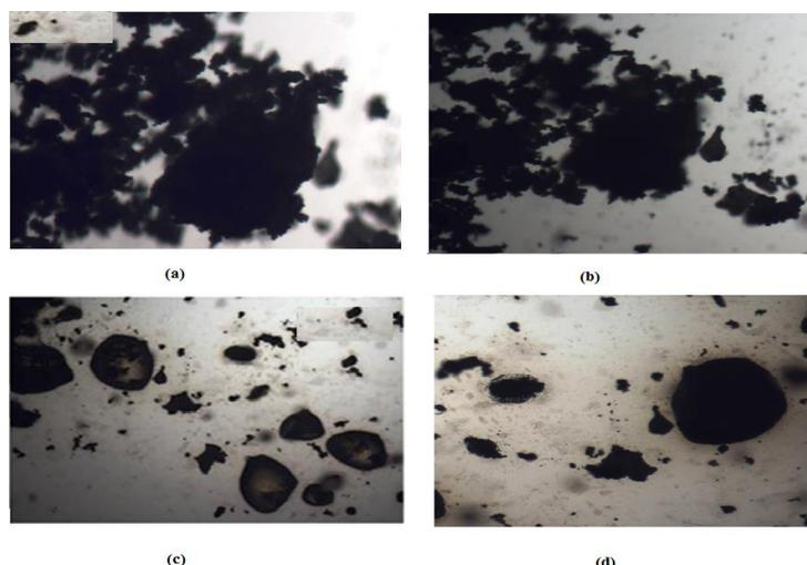
**Figure 15: ETNICA before melting (b) ETNICA starting to melt (c) ETNICA melting at 128.23°C (d) ETNICA fully melted**
