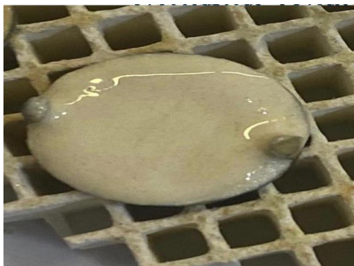
Figure 4 A base metal model covered with opaque porcelain layers and dentin porcelain Super Porcelain EX -3, Tokyo, Japan) Noritake
