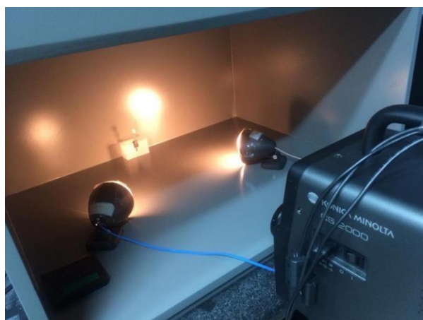
The samples' color was recorded on a white background using a spectrophotometer (Spectroradiometer Cs-20000-Konica Minolta, Berlin, Germany)
