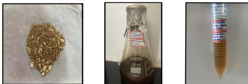
FIGURE 1: Preparation of Bionanocomposite - tamarind seed mediated silver nanoparticles with chitosan.
