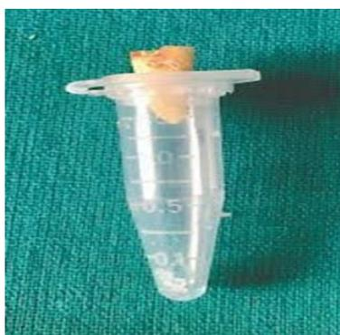
Teeth mounted in eppendorf microbalance tube
