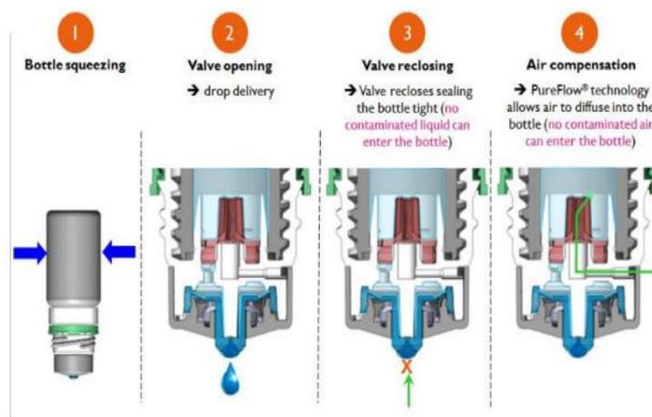
**FIG.1.** System functioning
