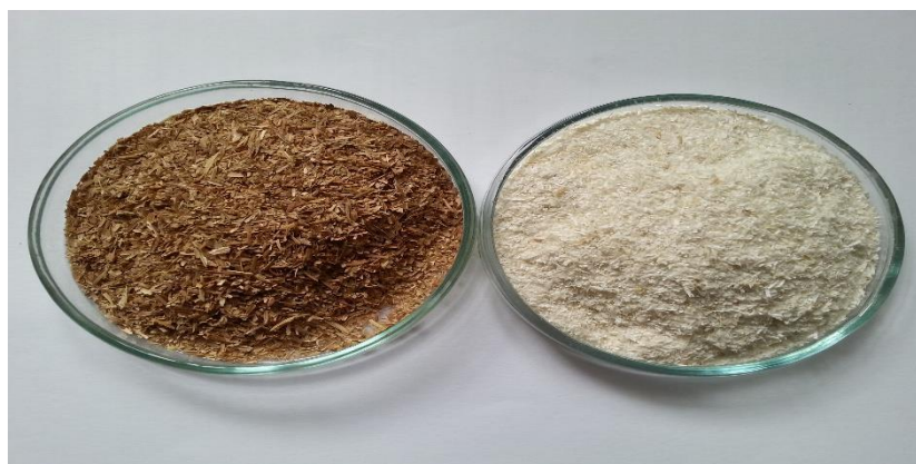
FIGURE 1: Rice husk, (Left) before pretreatment, (Right) after pretreatment
