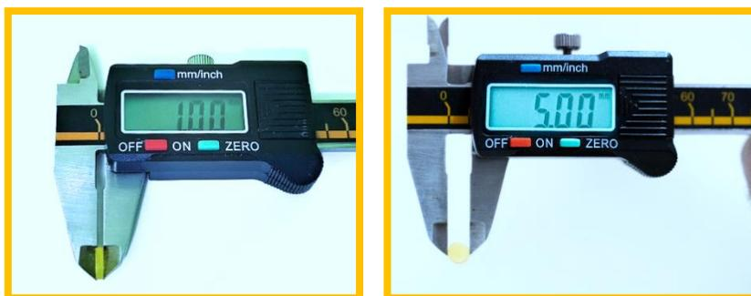
**FIGURE 1.** The bonding agents' discs after removal from the mold, confirming the dimensions (thickness and diameter) of the bonding agents discs.
